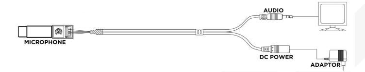
Remark: Since Hi sensitivity microphone, AA003PJA audio pick up box must be put at 5 meters away from monitor to avoid any audio reverberation.
